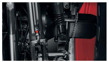
The front driven axle of the FORTERRA HSX and HD models can be optionally suspended. In combination with the suspended cab, this offers a smooth and comfortable drive.
